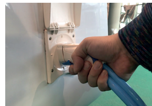
To remove, press the trigger with your index finger and pull towards you
