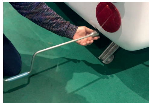
Insert winder into cut-out & connect with hexagonal nut
