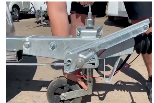
Wind jockey wheel up fully, lift & clamp into position
