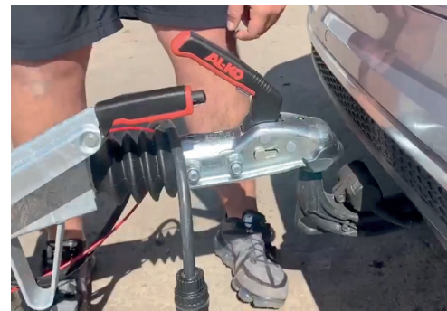
Wind jockey wheel down until coupling head connects with tow ball
